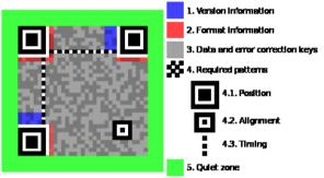
**b. High Capacity Encoding of Data** – As compared to 2D bar code, QR Code is capable of handling several dozen to several hundred times more information. QR Code is capable of handling all types of data, such as numeric and alphabetic characters, Kanji, Kana, Hiragana, symbols, binary, and control codes. Up to 7,089 characters can be encoded in one symbol. In the figure below it shows that a QR code symbol of this size can encode 300 alphanumeric characters.(Denso 2010)
