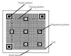
specific digital destination. Additional to the characteristics for two-dimensional symbols such as large volume data (7,089 numerical characters at maximum), high-density recording (approx. 100 times higher in density than linear symbols), and high-speed reading, QR Code has other superiority in both performance and functionalities aspects.
